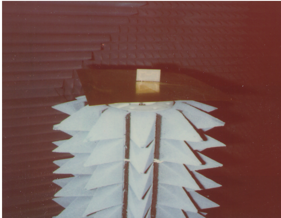
Figure 4.4: Photograph inside anechoic chamber zoomed in on fractal loop antenna on rotating pedestal.
